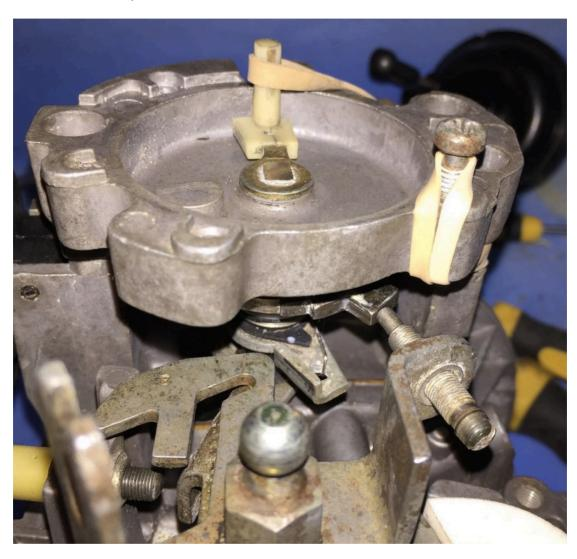
Push fast idle cam, or provide vacuum to pull-down unit, so that fast idle screw drops to next step on cam. Adjust choke flap gap by turning screw in
