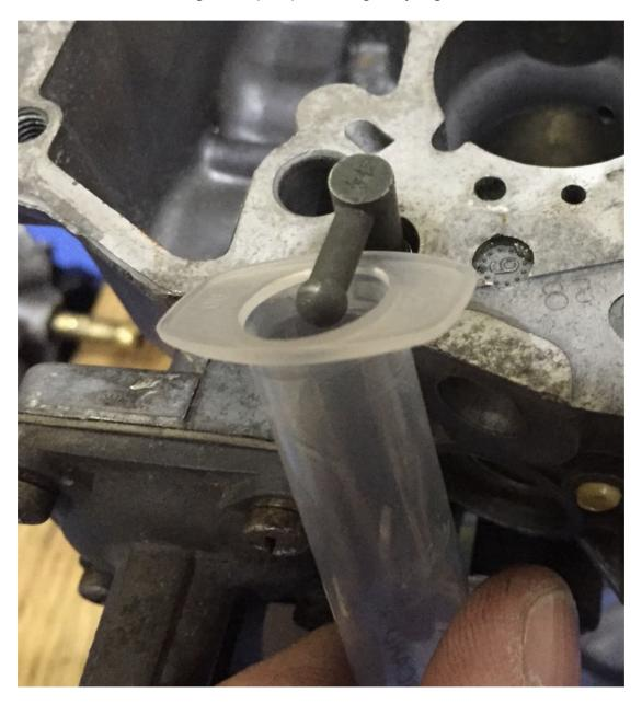
Adjust with cam – left for more, right for less. Possibly bend (straighten) pump arm to eliminate gap/slack
